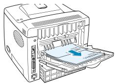
Printing from the Multi-Purpose Tray to the rear output tray provides the **straight paper path**. Opening the rear output tray might improve output quality with the following:
